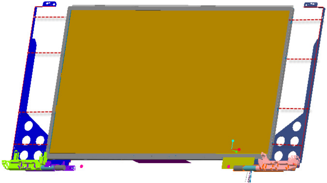
Figure 4-20-4 Remove the LCD hinge
