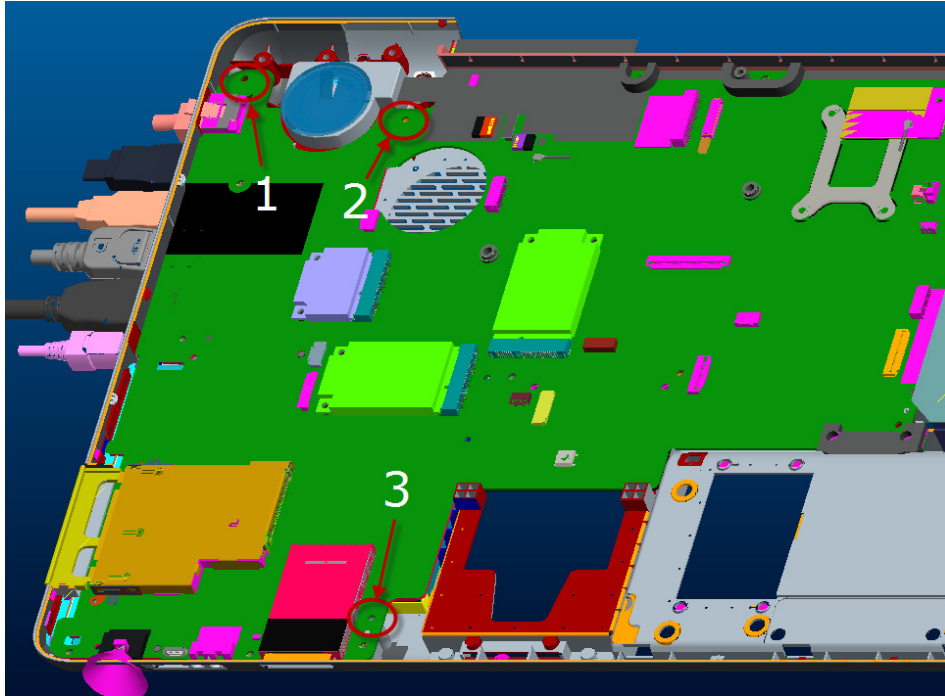
Figure 4-6-1 Remove an optical disk drive
